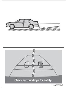
When the grade behind the vehicle slopes up sharply, objects appear to be farther away than they actually are.
