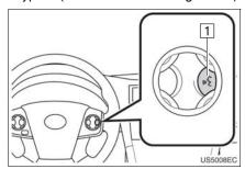
► Type B (Four direction steering switch)
