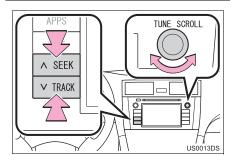
"SEEK/TRACK" button: Press the "^" or "V" of "SEEK/TRACK" button to select a desired track.
