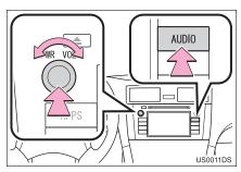
"AUDIO" button: Press this button to display screen buttons for the audio system.
