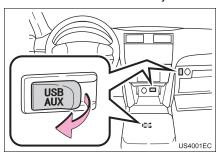
The USB/AUX port is located on the instrument panel, or in the console box or glove box etc. The location and design are different depending on the vehicle. For details, see the Pictorial index of "Owner's Manual". **2** Press the "APPS" button to display the "Applications" menu screen.
