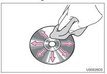
To clean a disc: Wipe it with a soft, lintfree cloth that has been dampened with water. Wipe in a straight line from the center to the edge of the disc (not in a circle).
