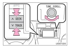
"SEEK/TRACK" button: Press the "^" or "V" of "SEEK/TRACK" button to select a desired file.
