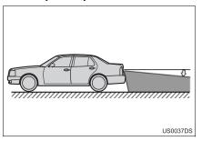
When any part of the vehicle sags due to the number of passengers or the distribution of the load, there is a margin of error between the guide lines on the screen and the actual distance/course on the road.
